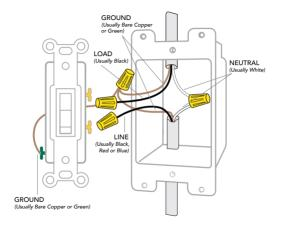
Turn the power back ON at the breaker. Using your voltage detector, identify which of the two wires you removed is energized. This is the "line" wire. The wire that is not energized is the "load" wire. Note these two wires for future reference.
