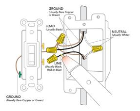
Turn the power back OFF at the breaker and install the iDevices<sup>®</sup> Dimmer Switch according to the diagram. Ensure all wire nuts are securely fastened.
