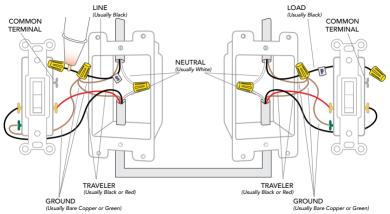
Install the iDevices® Dimmer Switches according to the diagram. Ensure the wire nuts are securely fastened.
