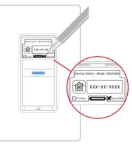
Extend the pull out tab on the front of the Dimmer Switch connected to the load wire (identified in step 5). Using a ballpoint pen, put an "X" in the box to indicate that this is the Primary Switch.
