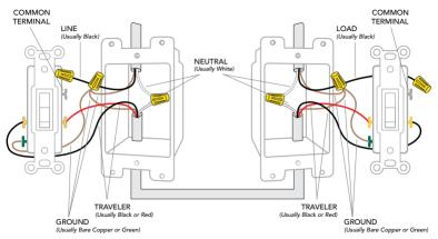
Turn the power back ON at the breaker. Using your voltage detector, identify which of the two wires you removed from the common terminal is energized. This is the "line" wire. Mark this wire as the <u>Secondary (S) Switch Position</u>. You will need to refer to this during the **Wireless Communication Setup**.
